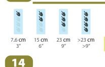
The depth gauge indicates the approximate depth of a buried target and has 4 levels in increments of nearly 7.6 cm (3"). The more 🔌 icons are shown on the LCD screen, the greater the depth of a possible buried item. The measurement accuracy depends on many factors such as the target type, soil conditions, etc.
