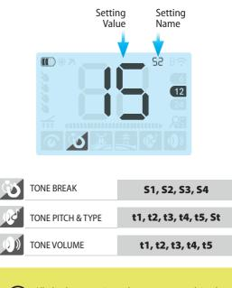
All the latest settings changes are saved in the memory of the device before it turns off.
